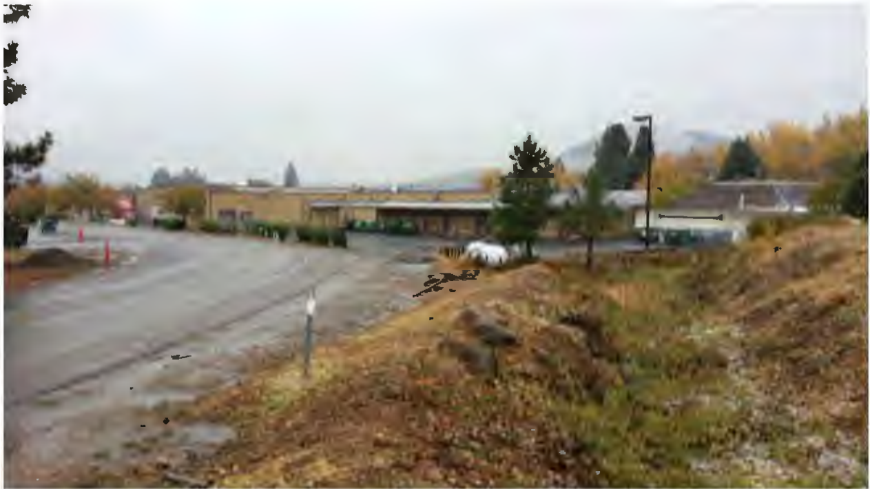
Figure 4-124 American Valley Localized Flooding – Strip Mall Containing Paradise Grill and other Businesses. Water can Overtop Earthen Ditch on Right, or Flow Down Street on Left when Storm Drain Floods behind Les Schwab
